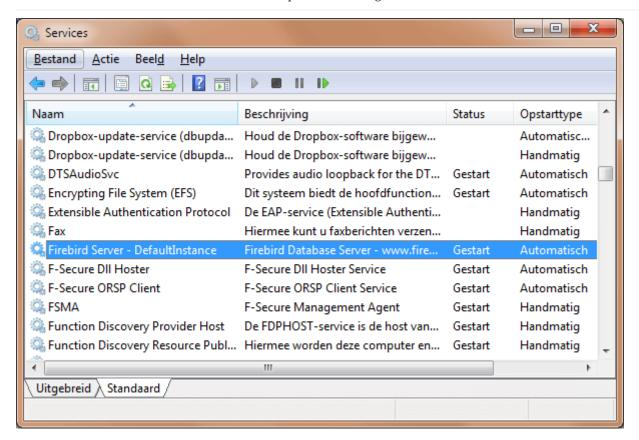
You should at least find the Firebird server in the services listing. The Guardian may or may not be running, depending on the choices you made during installation. If you didn't opt to start the server at the end of the installation process, you may do so now by right-clicking on the Firebird entry (or the Guardian) and choosing Start.
