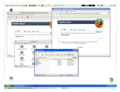
To enable seamless mode, after starting the virtual machine, press the Host key (normally the right control key) together with "L". This will enlarge the size of the VM's display to the size of your host screen and mask out the guest operating system's background. To go back to the "normal" VM display (i.e. to disable seamless windows), press the Host key and "L" again.
