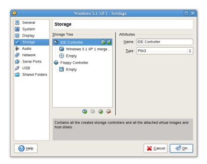
In a real PC, so-called "storage controllers" connect physical disk drives to the rest of the computer. Similarly, VirtualBox presents virtual storage controllers to a virtual machine. Under each controller, the virtual devices (hard disks, CD/DVD or floppy drives) are shown that are attached to the controller.
