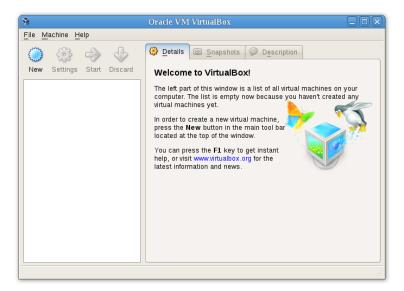
On the left, you can see a pane that will later list all your virtual machines. Since you have not created any, the list is empty. A row of buttons above it allows you to create new VMs and work on existing VMs, once you have some. The pane on the right displays the properties of the virtual machine currently selected, if any. Again, since you don't have any machines yet, the pane displays a welcome message.
