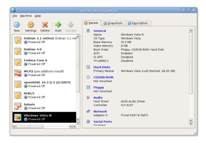
On the left, you can see a pane that lists all the virtual machines you have created so far (three in the example above). A row of buttons above it allows you to create new VMs and work on existing VMs. The pane on the right displays the properties of the virtual machine currently selected, if any.
