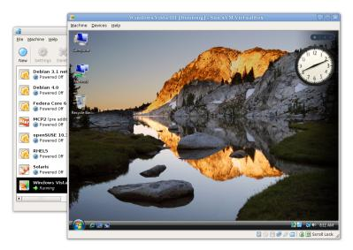
VirtualBox allows the guest code to run unmodified, directly on the host computer, and the guest operating system "thinks" it's running on real machine. In the background, however, VirtualBox intercepts certain operations that the guest performs to make sure that the guest does not interfere with other programs on the host.
